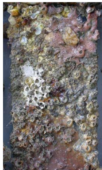
Biofouling after 3 months at marine immersion dock- May to August 2006
