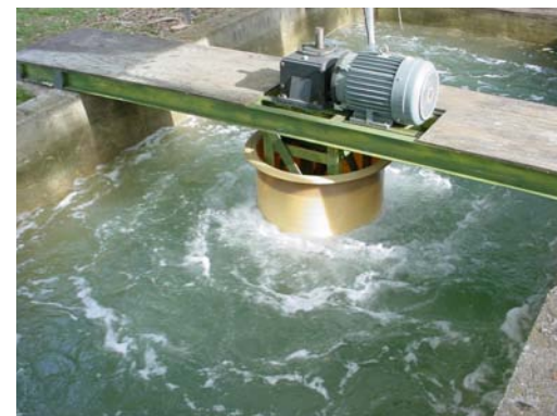
"Paint-Wheel" rotating at 16 knots during dynamic test of hull coatings
